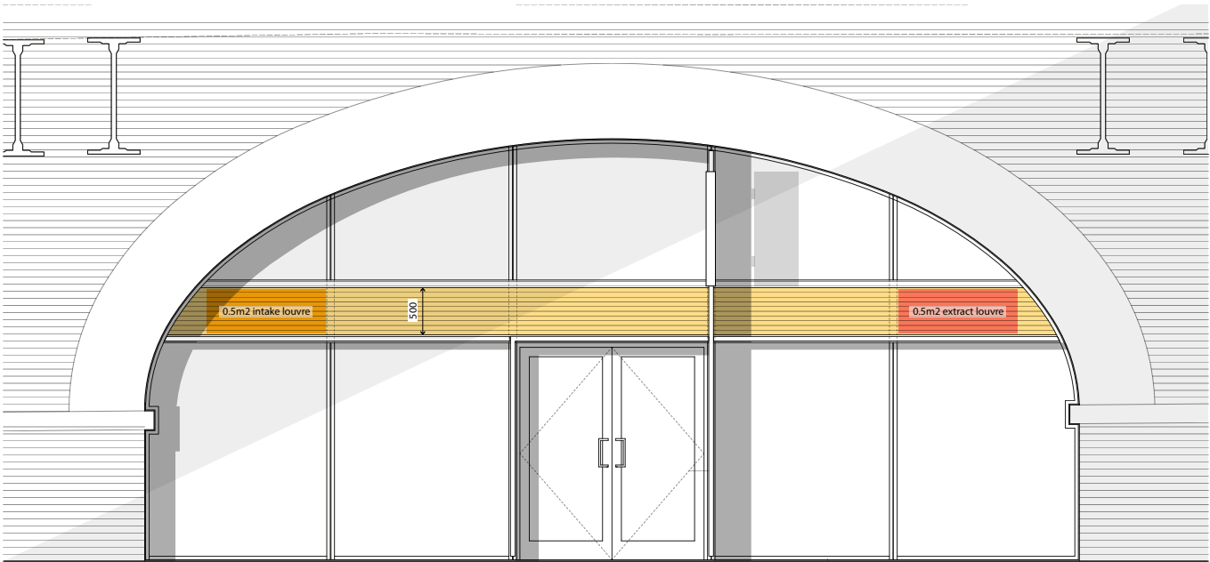
Fig 6.3.138: Elevation: Designated louvre zone for a typical A1 shopfront
