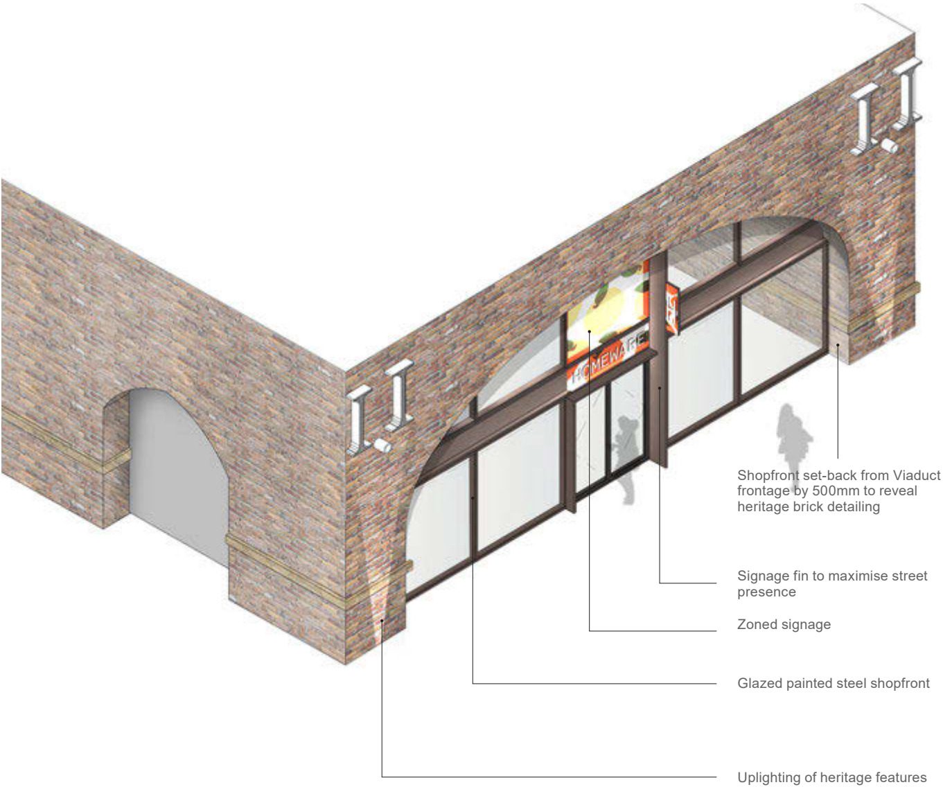
Fig 6.3.161: Axonometric of typical A1 shopfront
