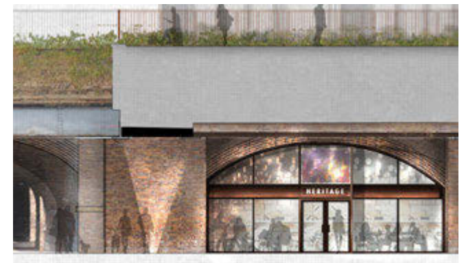
A3 (restaurant) Glazed painted steel shopfront with servicing support provided by additional louvre area in the cross arches
